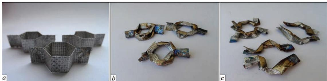
**Figure 4.** General view of samples of individual honeycombs before (*a*) and after mechanical compression tests (*b*)
