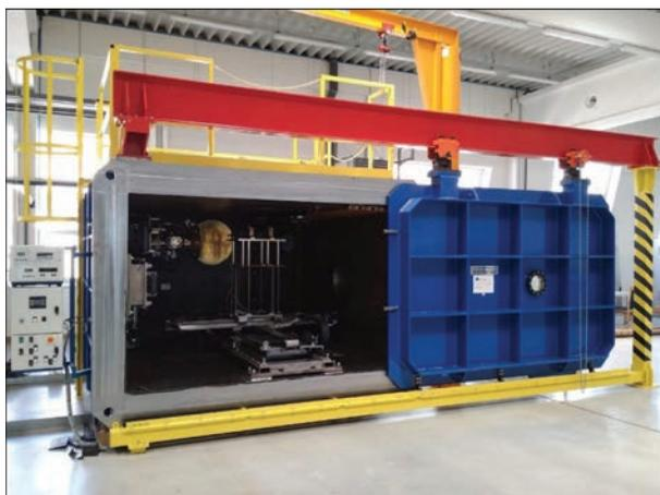
Figure 1. PZ EZ 30 STU electron beam welding machine
