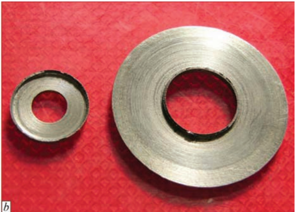
Figure 9. Scheme of the sample and assembly for ODS-steel tensile tests (a) and the view of the ODS-steel samples after the tests (b)
