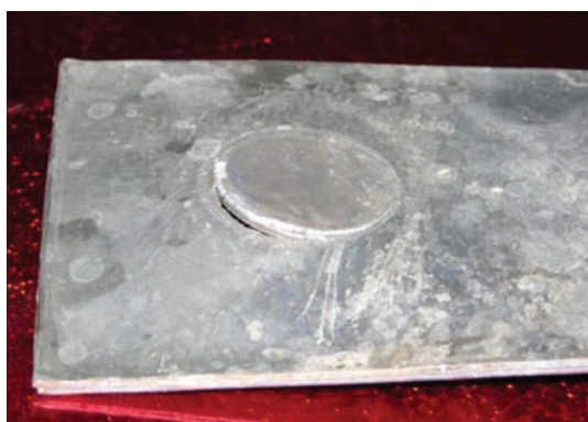
Figure 4. Plate welded with disks made of ODS-steel after EW
