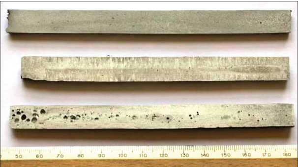
Figure 6. Macrostructure of the longitudinal section of rods with different nitrogen content, %: 1 — 0.73; 2 — 0.74; 3 — 0.9
