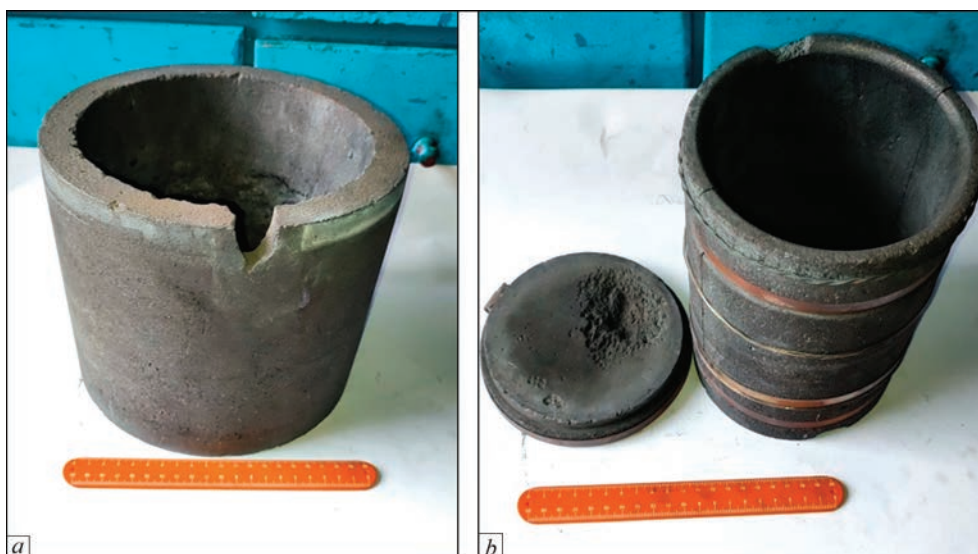
Figure 7. Appearance of graphite crucible (a) and permanent mould (b) for vacuum-arc remelting
