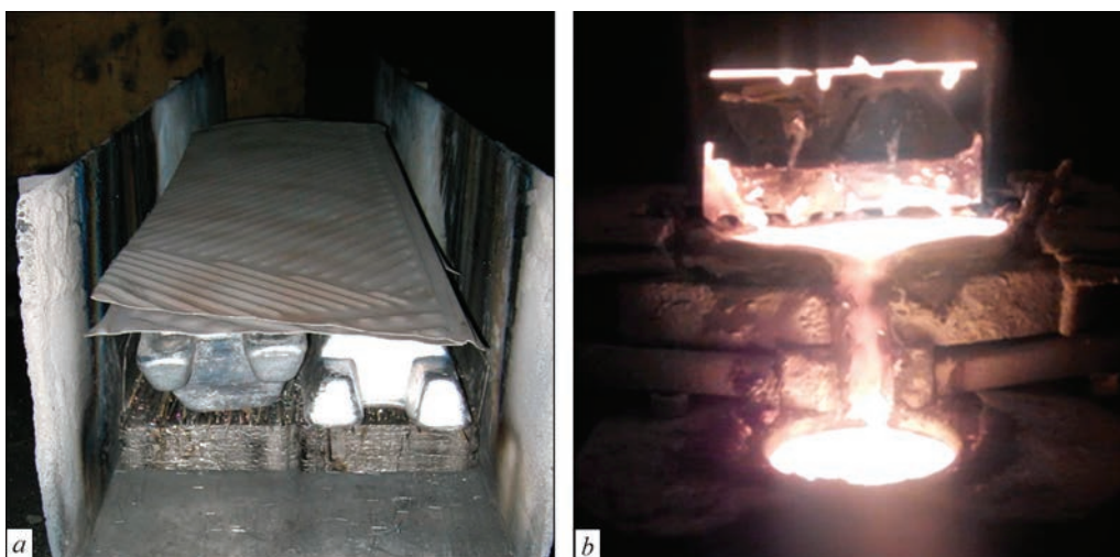
Figure 3. Charge billet (a) and electron beam melting process (b) of titanium aluminide ingot Ti-28Al-7Nb-2Mo
