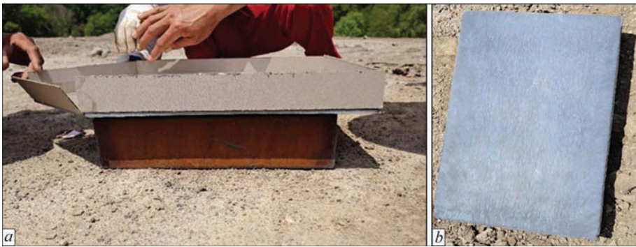
Figure 1. Appearance of plates of titanium alloy Grade 12 and carbon steel 09G2S before explosion welding (a) and after it (b) of the joint of TA10 + 09G2S bimetal produced by explosion welding.
