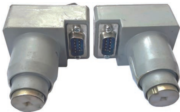
Figure 8. Images of the four-pole transducers for measurements of surface and subsurface stresses
