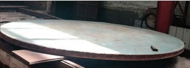
Figure 7. Appearance of TA10-09G2S bimetal tubesheet of 3340 mm diameter after heat treatment
