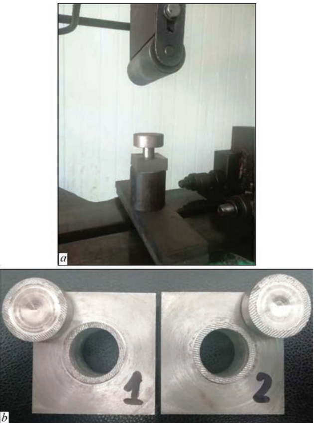
Figure 4. View of tear tests of the cladding (a) and of samples after testing for 6 mm cladding (b)
