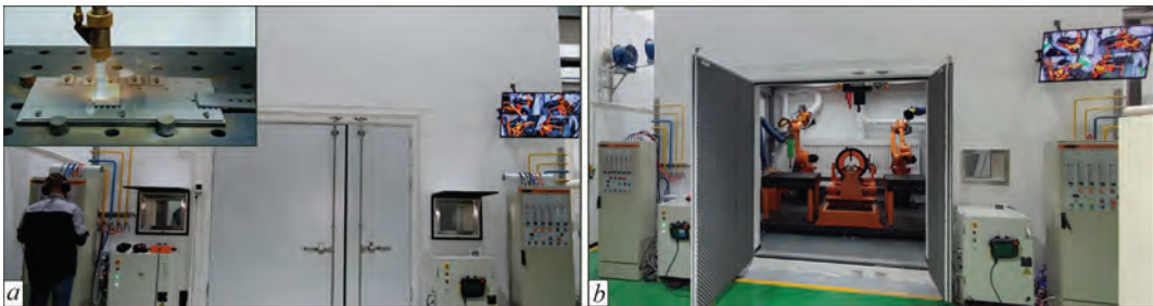
Figure 10. Rotobotic section of detonation gas spraying with realization of cumulative energy effect in MCDU, fitted with 6 axis robot with maximal arm range of 2238 mm and two-axis manipulator for rotation of the sprayed parts
