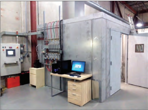
Figure 8. Section for detonation spraying of coatings
