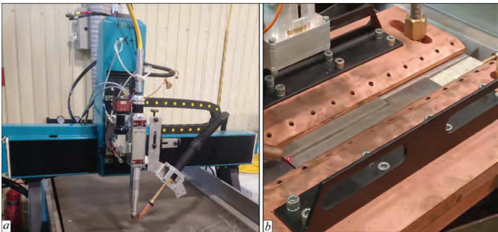
Figure 1. Facility ( a ) for conducting experiments on laser-P-MIG welding and clamp ( b ) with the sample after welding
