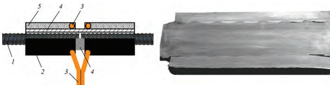
Figure 9. Principal scheme and macrosection of rebar joint made by explosion: 1 — rebar; 2 — charge shell; 3 — initiating detonating cord; 4 — coupling; 5 — explosive substance
