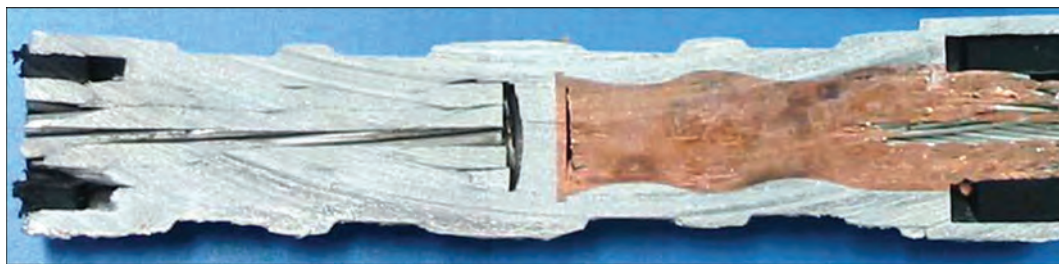
Figure 6. Joining of copper and aluminium cables by crimped couplings
