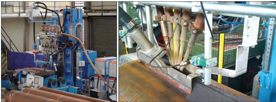
Figure 1. Five-wire SAW test stand for welding sheets and tubes at Fraunhofer IPK in Berlin (left) and multi-wire SAW welding head (right)
