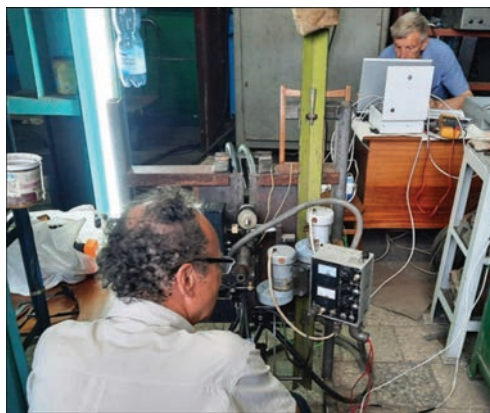
Figure 4. Submerged arc welding of vertical joint of 20 mm thick with forced formation
