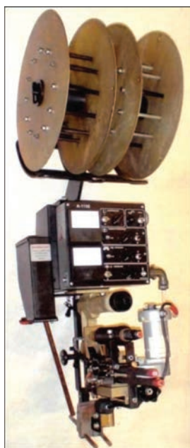
Figure 2. Appearance of prototype of mounting apparatus for welding vertical joints
