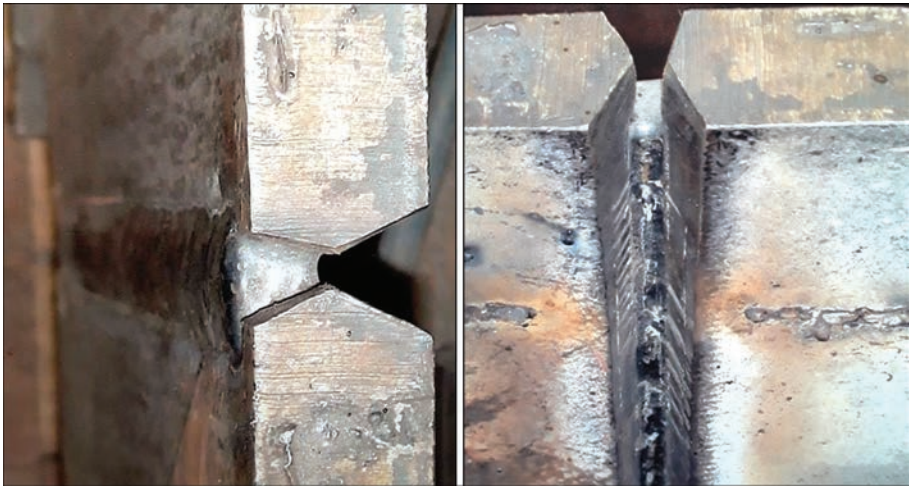
Figure 8. Appearance of weld after the first pass on the metal of 40 mm thick
