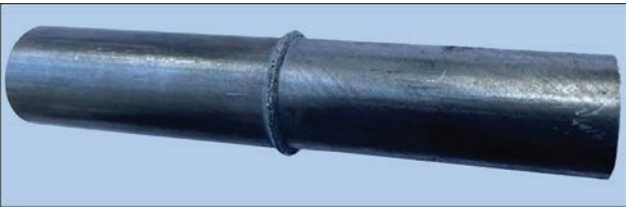
Figure 4. Welded joint of a pipe of Ø38×3 mm ing procedure recording was further developed into the welding procedure specification (WPS). Figure 6 gives the specification of the welding procedure, developed for Ø38×3 mm pipes from 09G2S steel.
