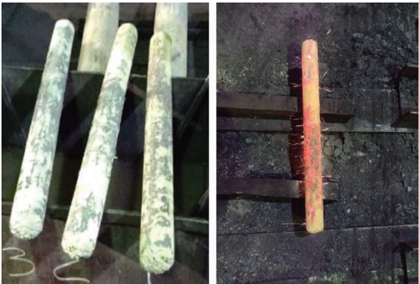
Figure 7. Appearance of 59 mm dia forgings of 60Zr–20Ti–20Nb alloy
