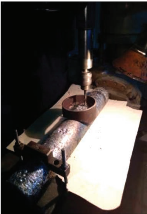
Figure 5. Selection of samples from 110 mm dia ingot of 60Zr-20Ti-20Nb alloy
