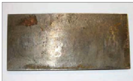
Figure 6. Sample of the ODS-steel + ODS-steel obtained by EW
