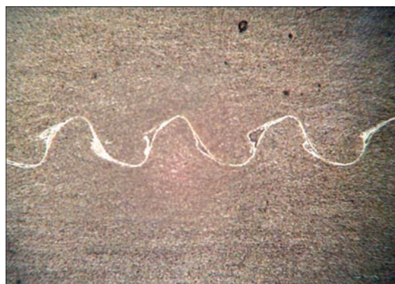
Figure 7. The microstructure of the EW zone of ODS-steel plates
