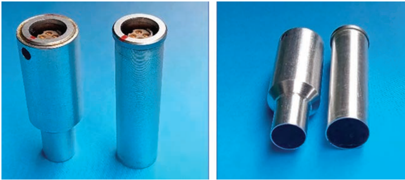
Figure 3. Studied double differential MDF 0801 and MDF 1001M type ECPs
