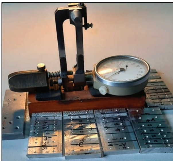
Figure 1. Appearance of mechanical strain gauge on a 20 mm base and cut-out parts of welded specimen (templates) with measuring bases (conical holes) for determination of residual stresses
