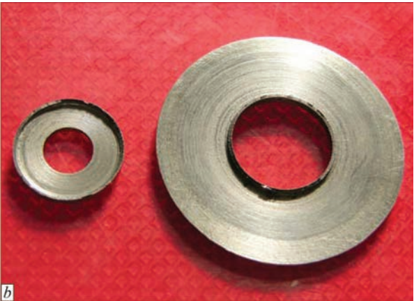
Figure 9. Scheme of the sample and assembly for ODS-steel tensile tests (a) and the view of the ODS-steel samples after the tests (b)
