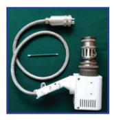
The universal electron beam gun, which is the basis of the welding tool, is capable of working both manually (when used by an astronaut-welder) and automatically as part of a robot.
