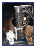
Additive technology is being developed with application of an electron beam gun with a wire feed mechanism in a vacuum chamber for repairing damage to space objects.
