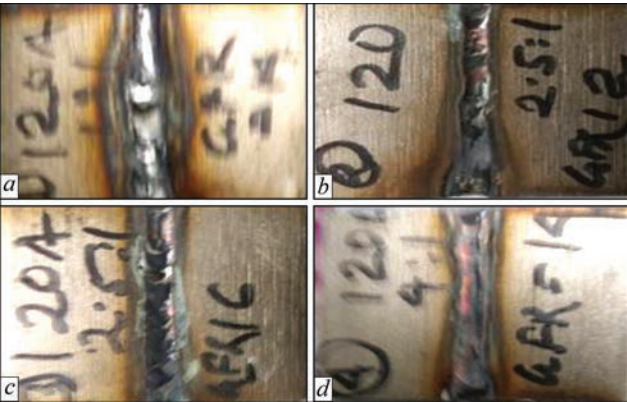
Figure 2. A-TIG welded specimens corresponding to respective experimental runs: a — weld joint in experiment 3; b — weld joint in experiment 9; c — weld joint in experiment 10; d — weld joint in experiment 12
