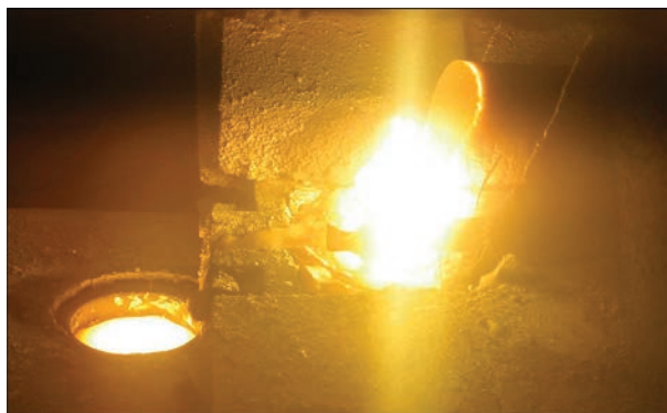
Figure 3. Melting process of an ingot with a diameter of 110 mm made of ortho-titanium aluminide Ti-39Nb-16Al-2.6Mo-1.4Zr alloy
