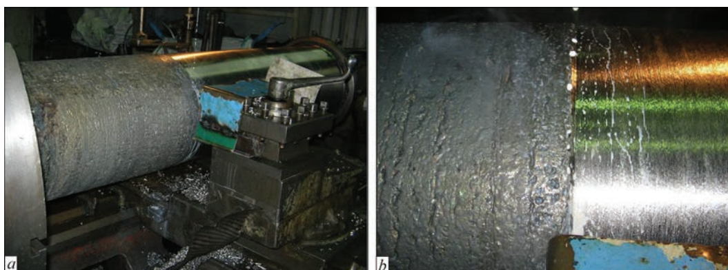
Figure 9. Machining of 400 mm dia. ingot from heat-resistant KhN60VT alloy
