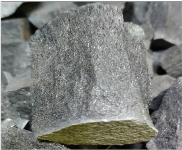
Figure 3. General view of a layer of slag in section (below is the slag-metal interface)
