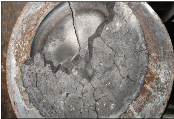
Figure 2. Appearance of slag and ferroalloy in the mould crucible. The overall weight of the melting products was 23.05 kg, of which 7.15 kg were ferrovanadium and 15.9 kg were slag (2.22 kg of slag per kilogram of metal). Evaporation losses were 0.55 kg. The quantity of the produced ferrovanadium is equal to 84.3 % of the total calculated quantity of vanadium and iron in the charge. Here, the specific power loss is equal to 1.958 kW·h/kg or 14 kW·h per one experiment.
