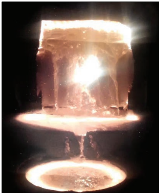
Figure 6. Melting of slag contained in the initial charge billet and up to 2000 mm length were produced as a result of the conducted melting operations (Figure 7).
