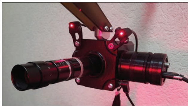
Figure 2. Appearance of shearography interferometer with laser modules and replaceable lens
