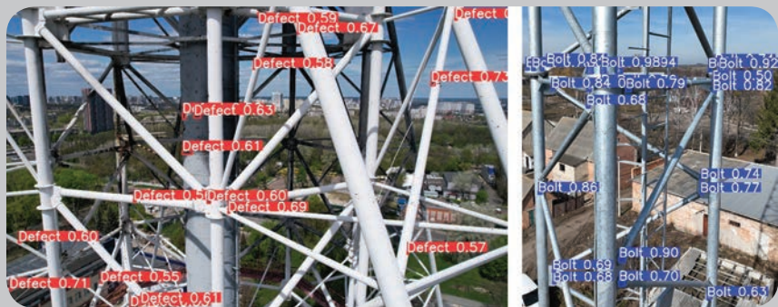
Detection results: AI-identified defects and bolts
