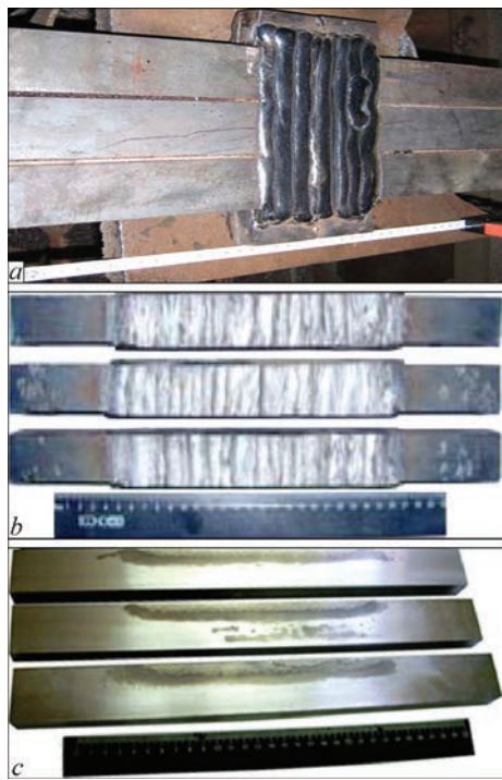
Figure 1. The blank package after surfacing (a), specimen blanks after cutting (b), specimens after final grinding (c)
