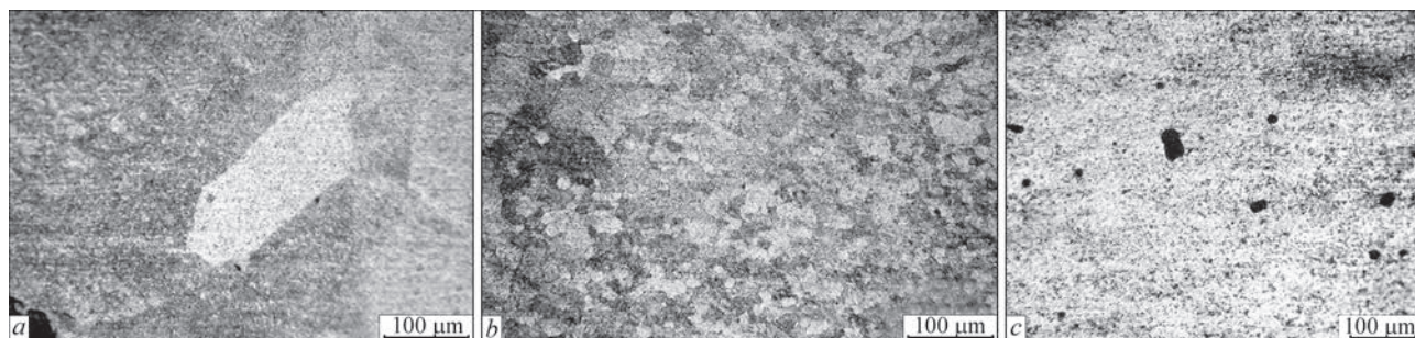
Figure 5. Typical structure of weld metal ( a ), HAZ metal ( b ), base metal ( c ) ( \times 200 )
