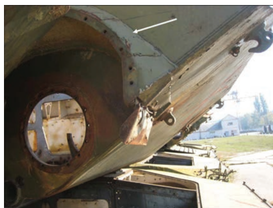
Figure 1. Fatigue crack in a welded joint of a LAV product after long-term operation
