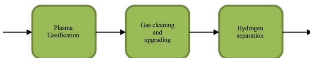
Figure 5. General technological scheme of hydrogen production by plasma gasification
