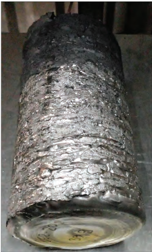
Figure 4. Ingot with a diameter of 110 mm made of ortho-titanium aluminide Ti-39Nb-16Al-2.6Mo-1.4Zr alloy
