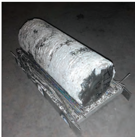
Figure 2. Charge billet for the production of ortho-titanium aluminide Ti–39Nb–16Al–2.6Mo–1.4Zr alloy
