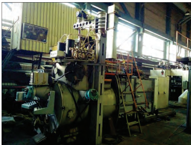
Figure 1. Laboratory electron beam UE-208M installation
