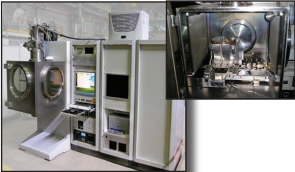
CB 112 mashine: 0.3 m³, 60 kV, up to 15 kW
