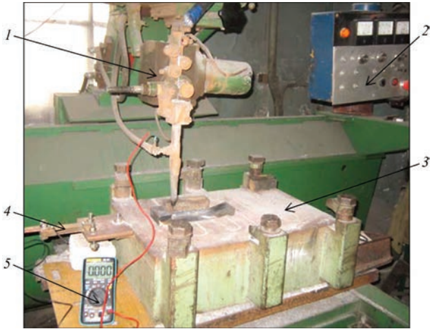
Figure 1. Appearance of the laboratory surfacing installation: 1 — welding automatic machine A-1406; 2 — control panel; 3 — welding table with a fixed test specimen; 4 — measuring shunt; 5 — digital self-recording ANENG AN9002 multimeter
