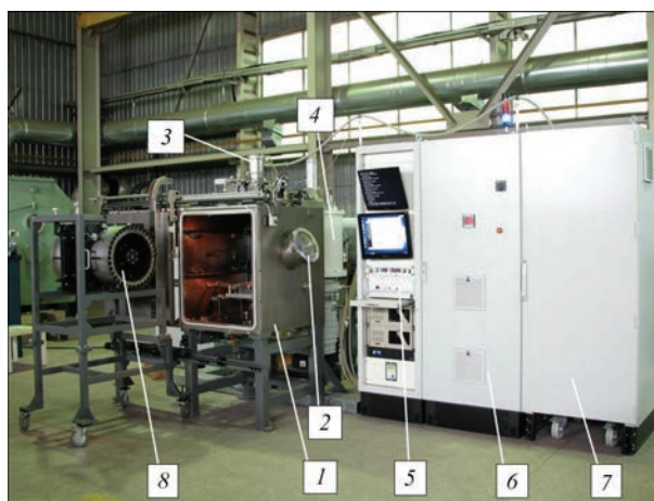
Figure 3. SV 229 installation for electron beam treatment: 1 — vacuum chamber; 2 — inspection port-hole; 3 — electron beam gun; 4 — vacuum system; 5 — control cabinet; 6 — power cabinet; 7 — cabinet of high-voltage welding power source; 8 — loading device for feed drums of parts
