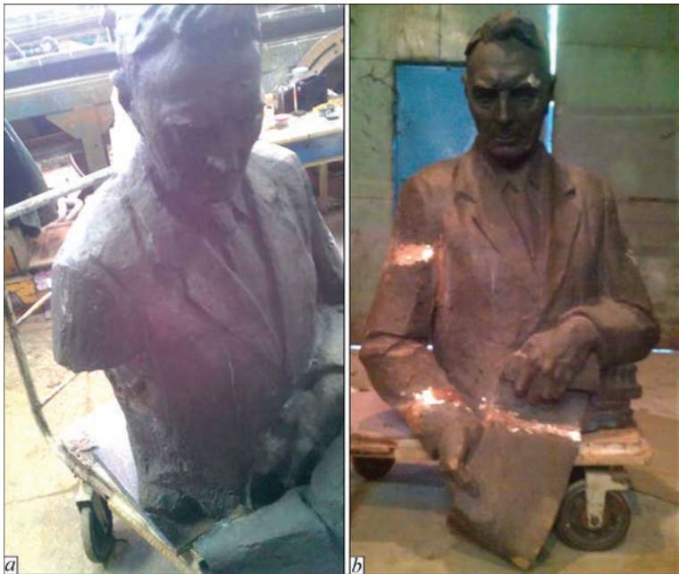
Figure 13. Monument to V.I.Tolubinsky with a broken off arm (a) and after coated electrode welding (b)
