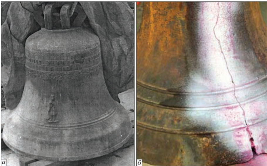
Figure 5. Appearance of a bell with the crack
