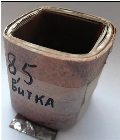
Figure 4. Pulsed magnet winding with 8.5 turns made from 60 \times 0.5 mm 2 strip along the height of 60 mm of 36 \times 36 mm 2 laminated core
