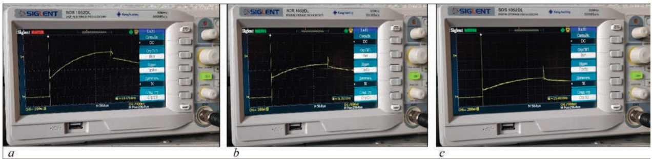
Figure 7. Current in the magnetization coil, equivalent to the magnetic field, when the key stage is powered by voltage of, V: a — 30; b — 20; c — 10. Magnetization pulse duration of 400 \mu s
