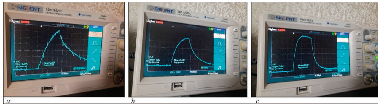
Figure 3. Signals equivalent to current in the pulsed magnet coils, depending on the number of turns of 1.2 mm wire in the core lower part: a — 15 turns; b — 9 turns; c — 6 turns
