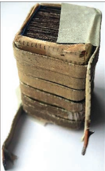
Figure 6. Model of a pulsed magnet with a coil made from 10 \times 1 mm 2 copper bus, 6.75 turns
