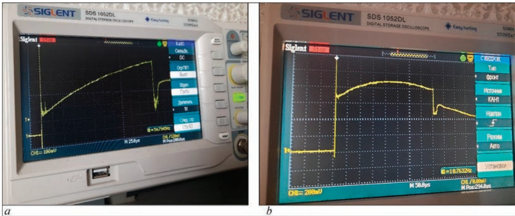
Figure 5. Voltage equivalent to current on 0.4 mOhm shunt with the pulsed magnet winding of: a — 8.5 turns from 60 \times 0.5 mm 2 strip; b — 5.75 turns from 60 \times 0.1 mm 2 strip. Supply voltage of the discharge key of 30 V
