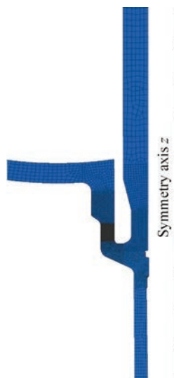
Figure 6. Finite element axisymmetric 2D model of welded joint No. 111
