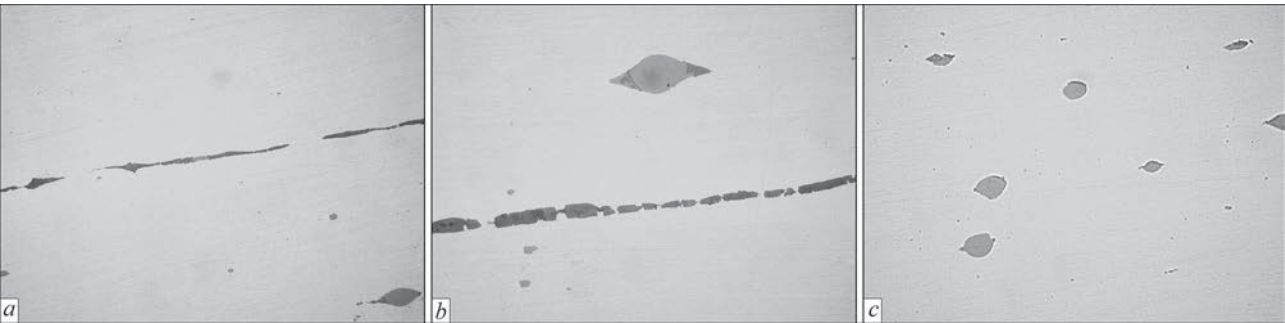
Figure 6. Lamellar silicates in steel: a — \delta = 15\text{ mm} , \times 500 ; b — chain of oxides in steel, \delta = 15\text{ mm} , \times 500 ; c — sulphides and oxysulphides near the fusion line, \delta = 15\text{ mm} , \times 500
