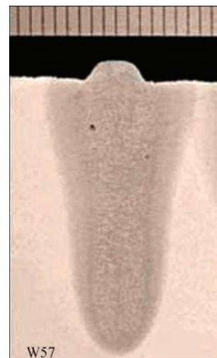
Figure 2. Weld produced in the flat position on low-alloy steel using a pulsed non-vacuum electron beam (NVEB), penetration depth 22 mm [7]
