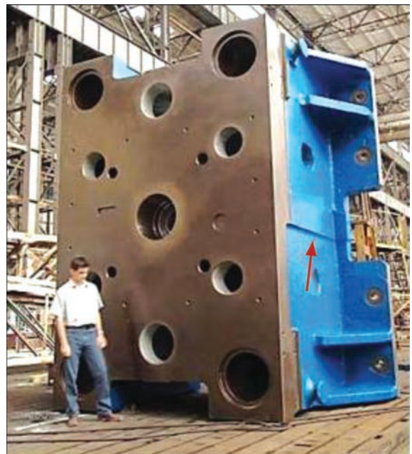
Figure 9. Welded blank of a hydraulic press crosshead. The blank weight is 150 t; the weld cross-section (indicated by the arrow), produced by ESW with a consumable nozzle, is 2490×3860 mm
