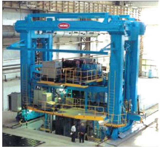
Figure 8. General view of the ESW installation with a consumable nozzle for joining metal, the weld cross-section of which can reach dimensions of 4000×6000 mm
