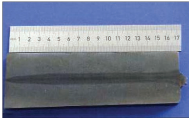
Figure 1. Macrosection of a welded joint produced by electron beam welding in vacuum [7]
