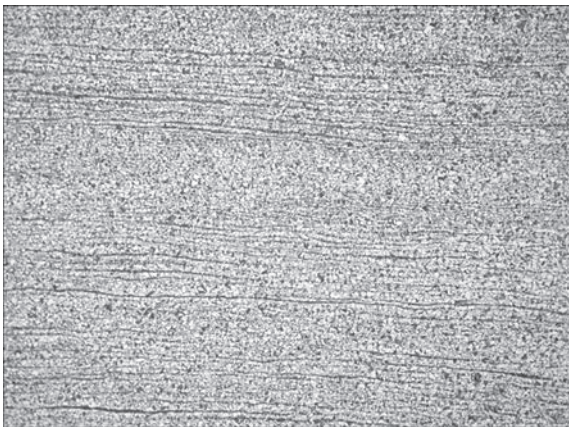
Figure 11. HAZ, full recrystallization zone ( \times 100 )
