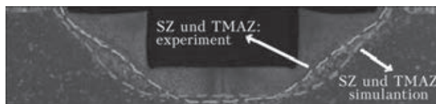
Figure 7. Comparison of experimentally and numerically determined thermo mechanical affected zone after FSSW of AA6082-T6 [11]
