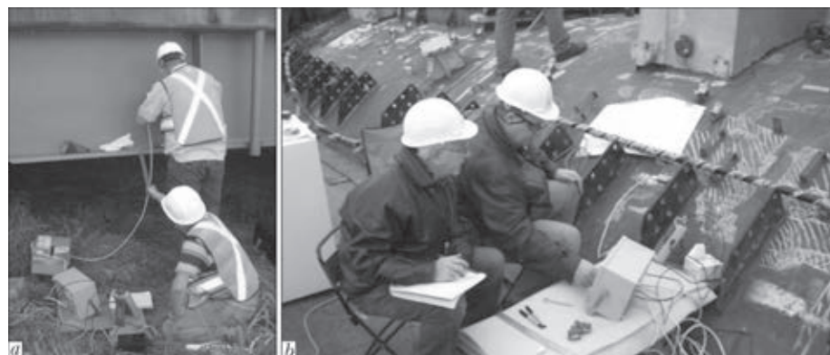
Figure 3. Application of the UltraMARS system for measurement of residual stresses in the zones of welded elements of a highway bridge (a) and a submarine pressure hull (b)
