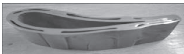
Figure 10. Turbine blade with complicated inner cooling gas channeling to be fabricated by additive manufacturing using electron beam physical vapor deposition (EB-PVD)
