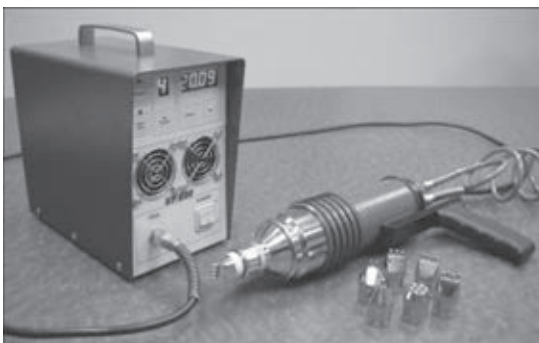
Figure 5. Advanced compact equipment for UIT/UP of materials, parts and welded elements
