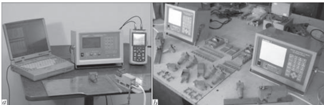
Figure 1. Ultrasonic Computerized Complex for residual and applied stress measurement: a — UltraMARS® model shown with a laptop and an oscilloscope; b — Next generation UltraMARS®-7 model shown with all transducers, transducer holders and attachments
