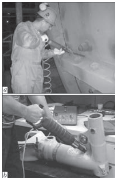
Figure 8. Examples of application of the UltraPeen system for fatigue improvement: a — of grinding mill when over 250 meters of welds were treated, b — of landing gear where critical from the fatigue point of view zone was treated
