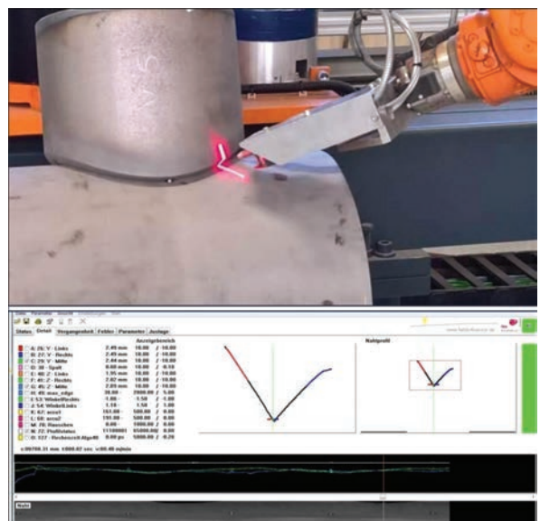
Fig. 3. Sensor arrangement and weld tracking recording on a T-joint before welding the root
