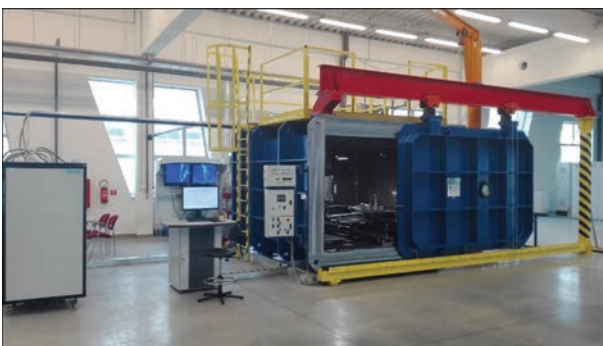
Fig. 13. The welding workplace type PZ EZ 30 TWINBEAM
