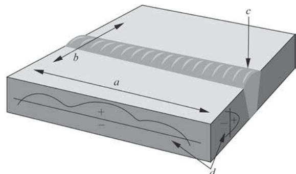
Fig. 1. RS induced by welding: a – longitudinal shrinkage; b – transverse shrinkage; c – weld seam; d – stresses
