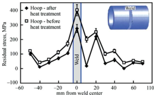
Fig. 4. Hoop RS (5 mm depth) determined by ND in a 2.25 Cr1Mo ferritic arc welded pipe before and after relaxation heat treatment
