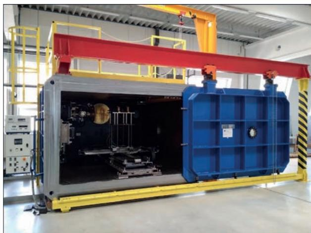
Fig. 1. PZ EZ 30 STU electron beam welding machine
