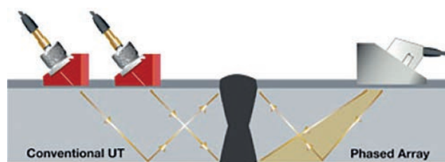
Fig. 9 Conventional versus phased array ultrasonic testing (courtesy Olympus)
