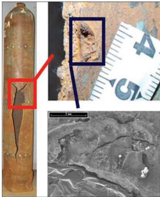
Fig. 1. Photo of a 40-liter oxygen cylinder made of 35G steel after hydrostatic testing with defect on the cylinder and crack viewed from above — from the outer surface of the cylinder
