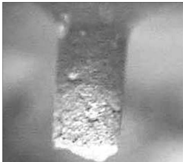
Figure 8. End face of the electrode with protruding NRI (melt No.1)
