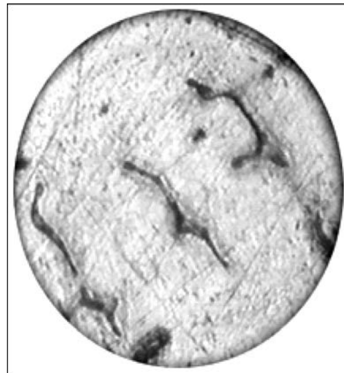
Figure 12. Formations of \delta -ferrite in microstructure of steel C20 (×200)
