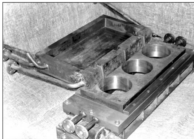
Figure 2. Technological equipment for simultaneous melting of several ingots
