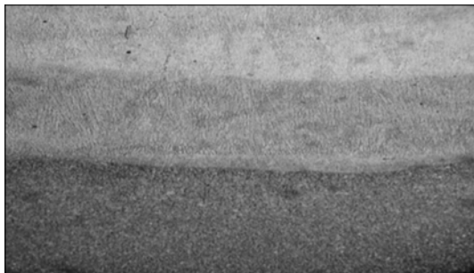
Figure 11. Microstructure of metal produced by method of two-layer multi-electrode (10 electrodes) surfacing of wheel rim using welding wire Sv-08KhM of 3 mm diameter and flux AN-60 ( \times 40 )
