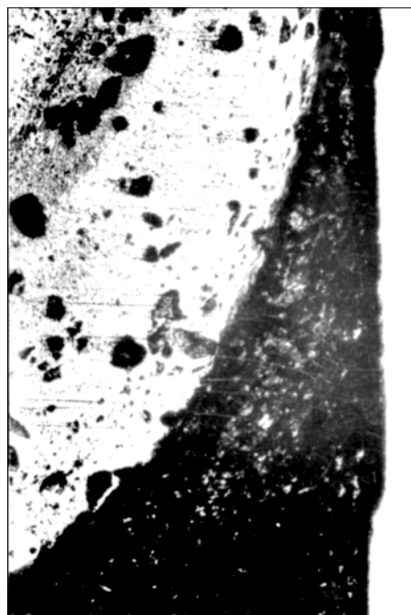
Figure 3. Area of the second zone (light, porous) abutting on third one (dark) ( \times 50 )
