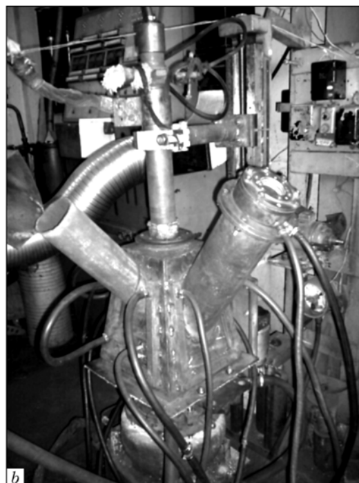
Figure 4. Scheme (a) and general view (b) of pilot installation: 1 — hollow electrode; 2 — mechanism for displacement of electrode; 3 — insulator; 4 — side panel; 5 — side panel cooling; 6 — plasma; 7 — power source; 8 — copper water-cooled mould; 9 — graphite crucible; 10 — metal ingot; 11 — molten metal; 12 — molten slag
