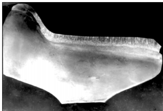
Figure 7. Microstructure of wheel renovated by method of multi-electrode surfacing
