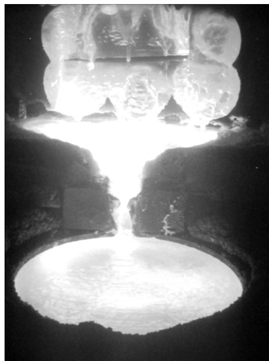
Figure 1. Melting of ingot from spongy titanium briquettes
