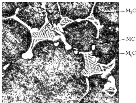
Figure 2. Morphology of eutectic in cast steel R6M5 (EBCHR) ( \times 1200 )
