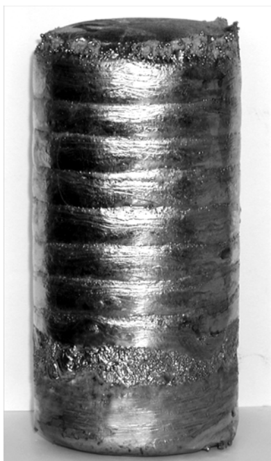
Figure 6. Appearance of ingot melted under the action of a pulsed longitudinal magnetic field ( t_{pulse} = 11 s, t_{pause} = 21 s, B = 0.21 T)
