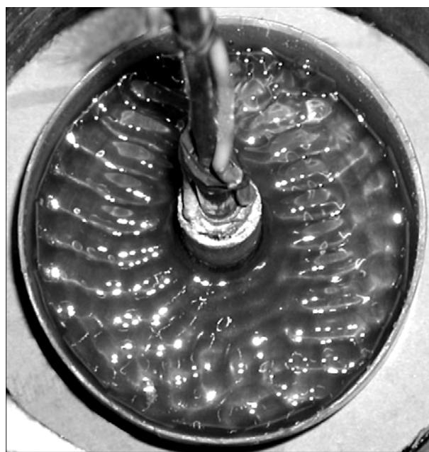
Figure 2. Vibration of a model liquid (concentrated solution of \text{CaCl}_2 ) under the action of longitudinal constant magnetic field at I = 40 \text{ A} , B = 0.2 \text{ T}
