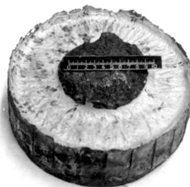
Figure 12. Casting-billet of 220 mm diameter with graphite rod produced in IRSM installation
