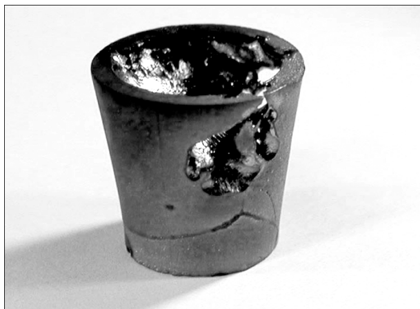
Figure 2. General view of crucible after melting
