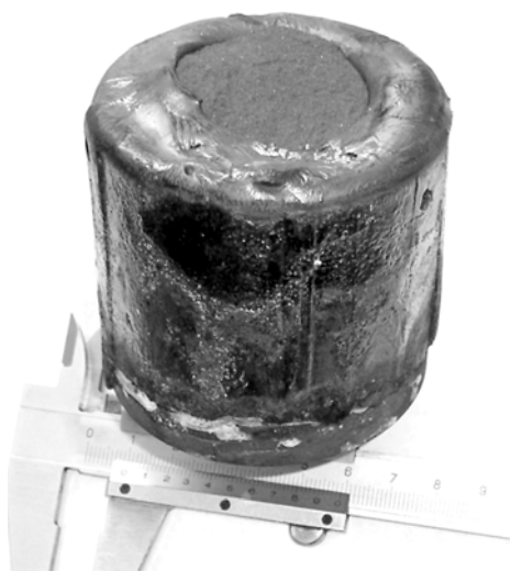
Figure 9. Appearance of hollow billet of 70 mm diameter with rod
