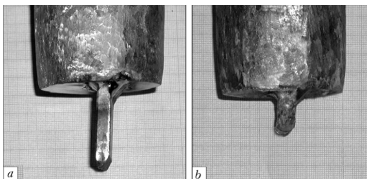
Figure 2. View of electrode end before (a) and after (b) melting of flux
