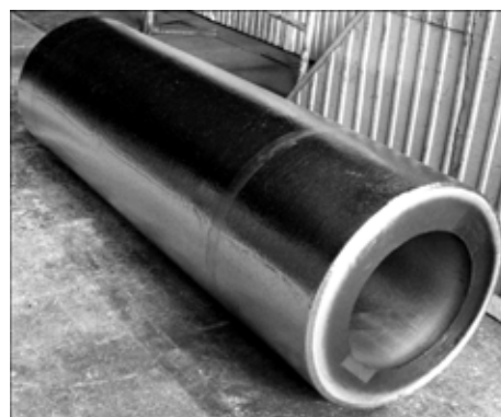
Figure 10. Pipe ingot of 600/400x2000 mm size
