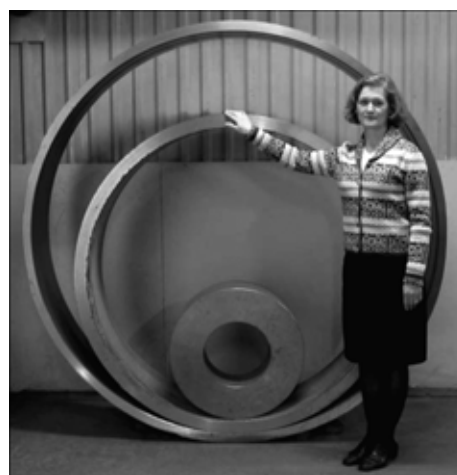
Figure 11. Expanded rings of 1850 and 1415 mm diameter
