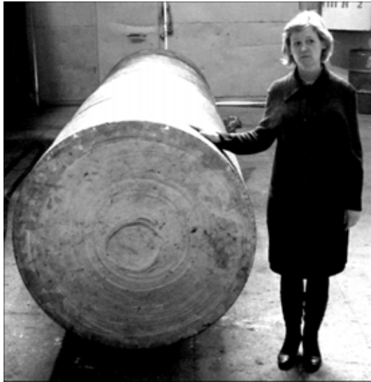
Figure 5. Ingot of 1100 mm diameter
