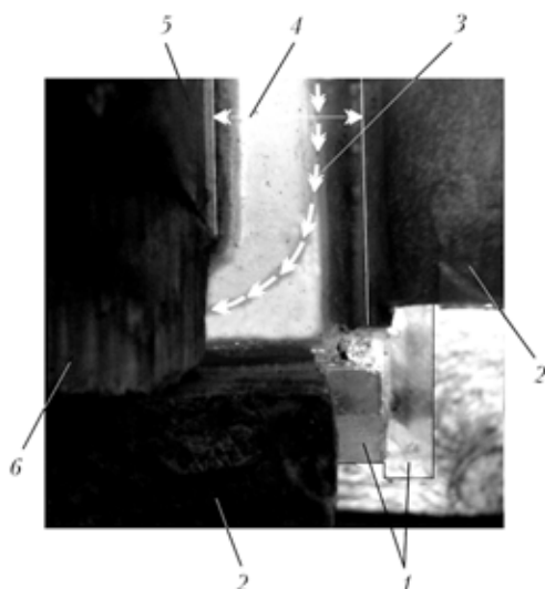
Figure 2. Rotation of horizontal flow in cladding in current-leading mould (view from above): 1 — walls of mould body; 2 — electrodes of current-leading section; 3 — flow of solution which models slag; 4 — spacing (17.5 mm); 5 — billet being clad; 6 — wooden distance bar
