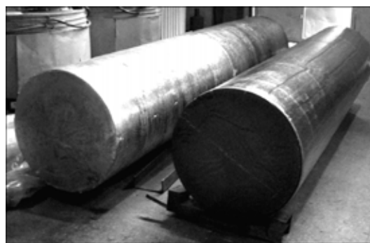
Figure 3. Flashed ingot of 850 mm diameter
