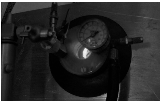
Fig. 3. Luminescent penetrant testing of aircraft constructions with vacuum appliance
