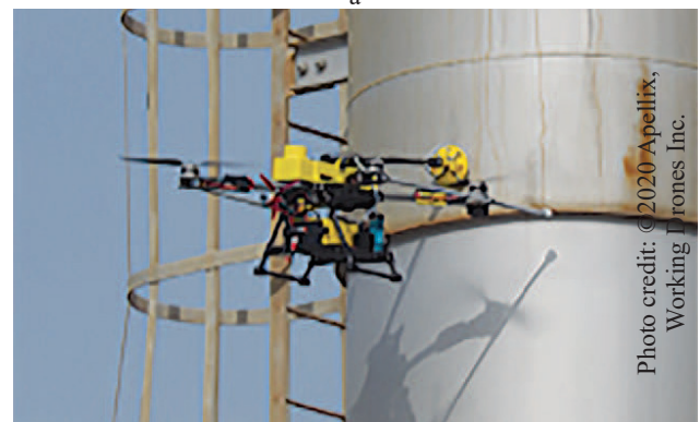
Figure 2. Ultrasonic thickness measurement system in action: (a) on an in-service aboveground storage tank; (b) on an in-service active flare stack.
