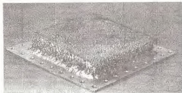
Figure 5. Welded model sample of a panel from 20 mm FA for thermal and sound insulation of engine compartment.
