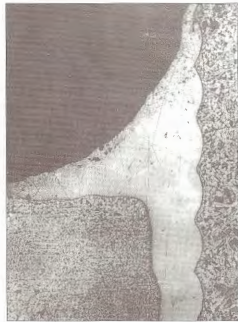
Figure 3. Microstructure of the brazed joint near the feed groove (x50 (reduced by 0.50)).
