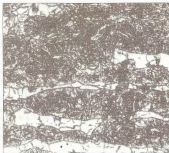
Figure 2. Structure of the steel 20Kh17N2 sample before hardening ( \times 600 ).
