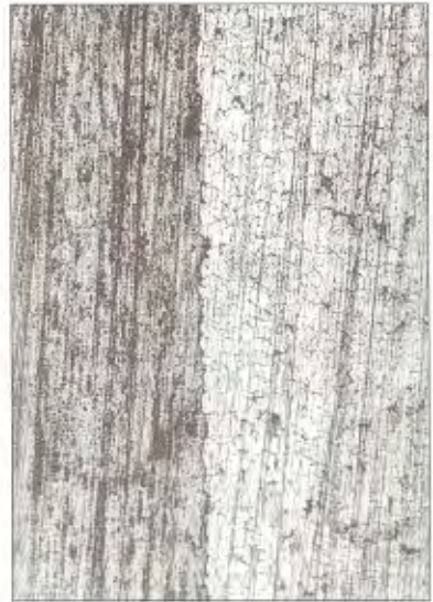
Figure 8. Microstructure of the joint between copper and metal-ceramic ( \times 100 ) (reduced by 0.80).
