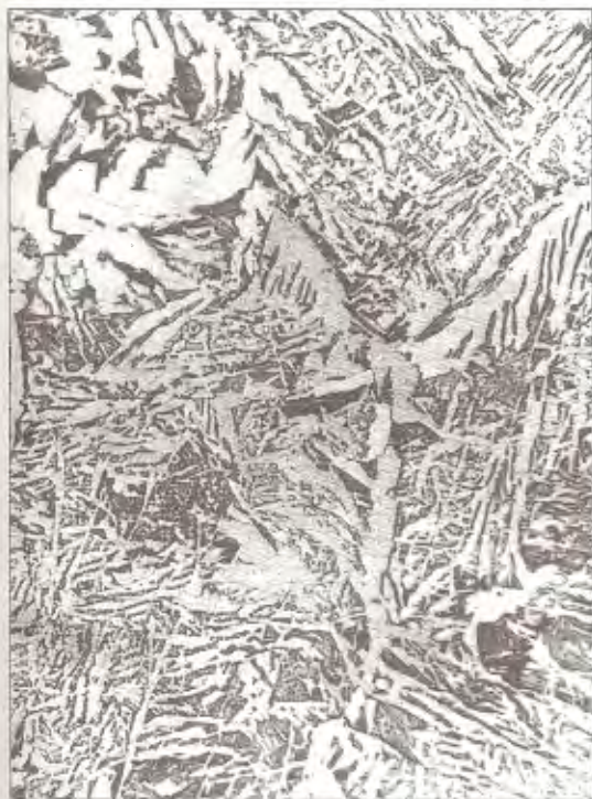
Figure 4. Microstructure of the zone of the joint produced by VDW with ~ 4 nm oxide thickness on the sample surface ( \times 200 ) reduced by 0.72)
