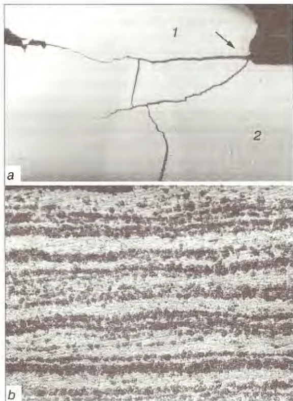
Figure 2. Lamellar-fatigue fracture of a refrigerating chamber: a — fracture site (shown by an arrow) (1 — stiffener; 2 — cylindrical case of a drum); b — ferritic-pearlitic banding of base metal ( \times 100 ) (reduced by 0.60)
