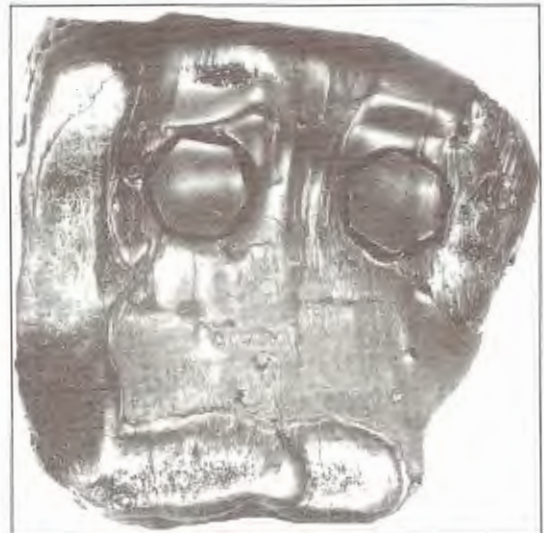
Figure 6. Asphalt mixer blade surfaced using the new PP-150Kh13R3F material after long-time operation
