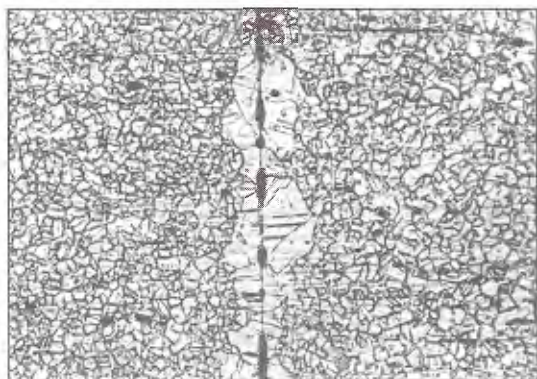
Figure 5. Microstructure of the bond in permalloy 50N ( \times 100 ) (reduced by 2/3 )
